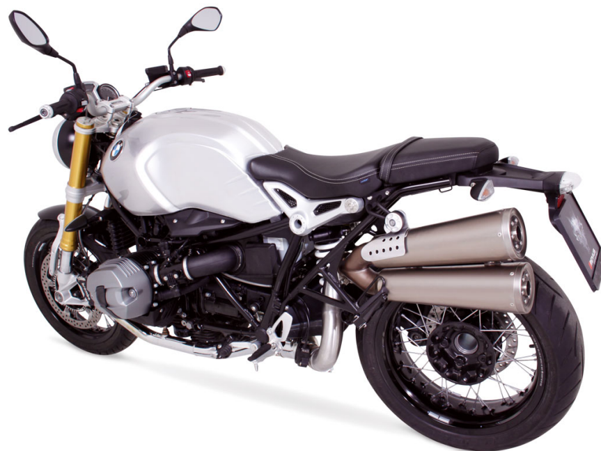
Upswept connecting tube with serial exhaust and heat shield
